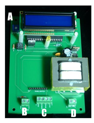
A-Display ContrastB-Solenoid Output (12 volts DC)C-Switch TerminalD-Power Terminal
