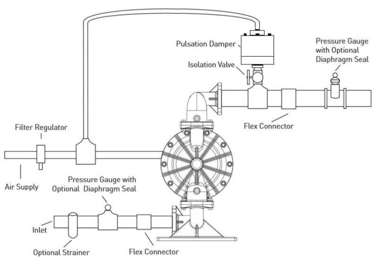
This illustration is a generic representation of an air operated double-diaphragm pump.
