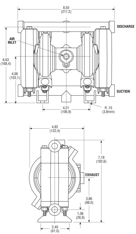
NOTE: AIR INLET IS ON THE SIDE WITH STAINLESS STEEL INSERT. THE AIR VALVE ASSEMBLY IS ON THE OPPOSITE SIDE OF THE PUMP.
