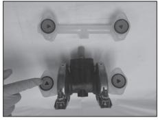
STEP 2 Remove the "Discharge Manifold".
