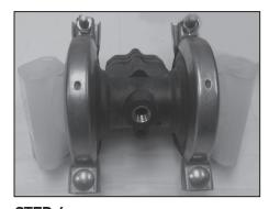
STEP 4 Set the "Intermediate" with attached "Outer Chambers" aside.
