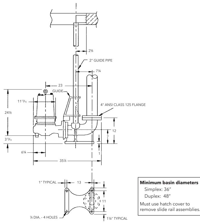
4NS/4XD ON A10-40 GUIDE RAIL - Submersible Sewage Pump
