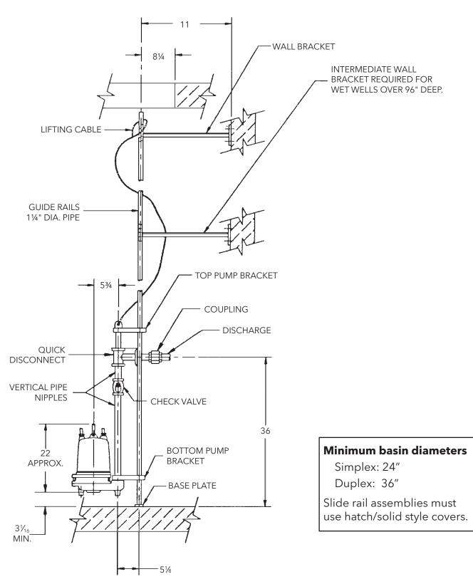
(All dimensions are in inches. Do not use for construction purposes.) \*\*To use catalog 1¼" Duplex Discharge Piping.
