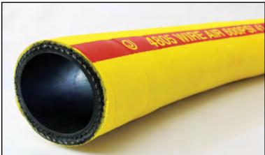
**CONSTRUCTION:** Tube is nitrile blend, smooth and black. Cover is SBR, yellow, fabric impression and pin-pricked. Reinforcement is two spiral wires.
