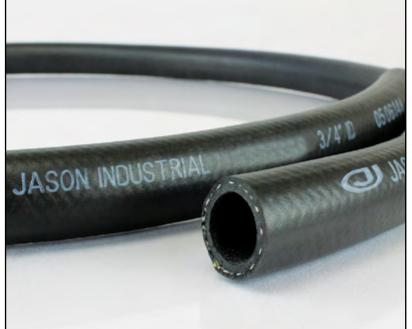
**CONSTRUCTION:** Tube and cover are TPR (NBR/PVC), smooth, high oil resistance, ARPM Class A. Cover is black Reinforcement is one braid, synthetic material.
