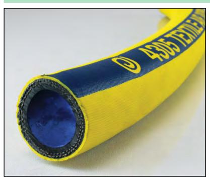
**CONSTRUCTION:** Tube is a nitrile blend, smooth and black. Cover is Nitrile/SBR, fabric impression, yellow, pin-pricked. Reinforcement is a two-ply synthetic fabric.
