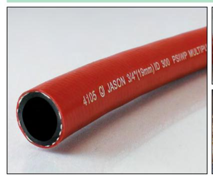
**CONSTRUCTION:** Tube and cover are TPR (NBR/PVC), smooth, high oil resistance, ARPM Class A. Cover is red. Reinforcement is one braid, synthetic material.
