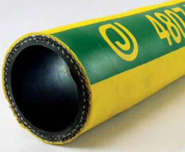
**CONSTRUCTION:** Tube is a hydraulic oil mist resistant, high heat synthetic rubber. Cover is EPDM, yellow, pin-pricked. Reinforcement is a two-spiral wire.
