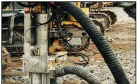
**CONSTRUCTION:** Abrasion resistant SBR tube and cover
