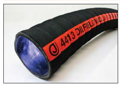
**CONSTRUCTION:** Tube is a nitrile blend blend. Cover is corrugated SBR blend. Reinforcement is a 4-ply high-tensile synthetic textile with a dual steel wire helix.
