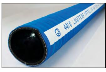
**CONSTRUCTION:** Tube is nitrile, black and smooth, ARPM Class A. Cover is CR, blue, corrugated, ARPM Class B. Reinforcement is a two-ply synthetic fabric with a double wire helix.
