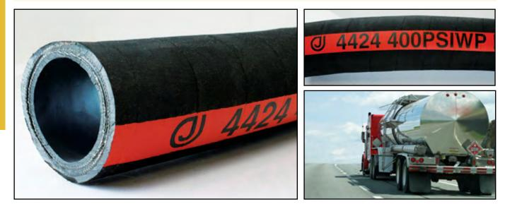
**CONSTRUCTION:** Tube is nitrile, black and smooth, ARPM Class A. Cover is CR, black, ARPM Class B. Reinforcement is a two-ply synthetic fabric with a dual wire helix.
