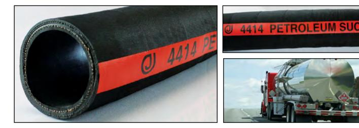
**CONSTRUCTION:** Tube nitrile, smooth and black. ARPM Class A. Cover is CR, ARPM Class B. Reinforcement is two-ply synthetic fabric with a dual wire helix.
