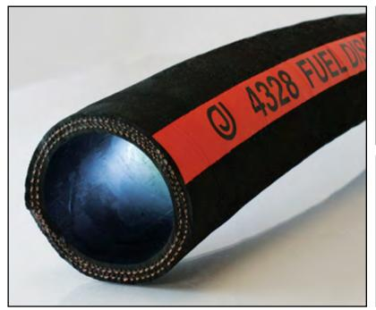
**CONSTRUCTION:** Tube is nitrile, smooth, ARPM Class A. Cover is CR, black, ARPM Class B. Reinforcement is two-ply synthetic fabric with a static wire.
