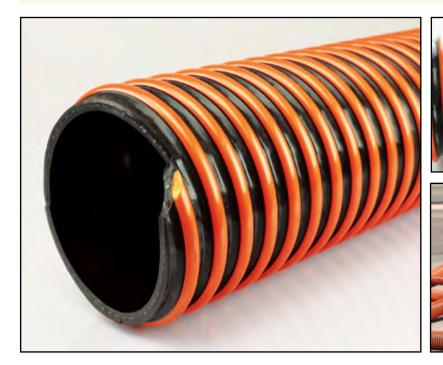
**CONSTRUCTION:** NBR/PVC tube, smooth bore with embedded SΩ ground wire in the hose wall with a sturdy clockwise PVC helix, one braid of high tensile polyester yarn reinforcement.
