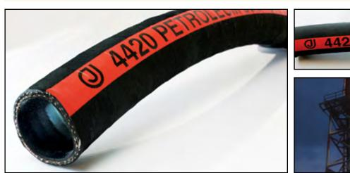
CONSTRUCTION: Tube nitrile, smooth and black. ARPM Class A. Cover is CR, ARPM Class B. Reinforcement is two synthetic plies with a dual wire helix. TEMPERATURE: -25°F (-32°C) to +200°F (+93°C)
