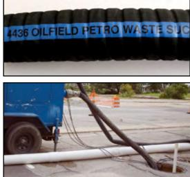
**CONSTRUCTION:** Tube is an NBR/SBR blend, black and smooth, oil resistant. Cover is an NBR/ PVC blend, black, flat corrugated w/ cloth impression, oil, abrasion, weather and ozone resistant. Reinforcement is a high tensile cord with a dual steel wire helix.
