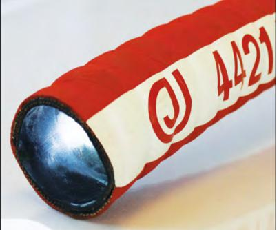
**CONSTRUCTION:** Tube is nitrile, smooth, ARPM Class A. Cover is CR, ARPM Class B, corrugated and red. Reinforcement is two synthetic plies with a wire helix.
