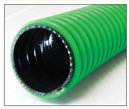
**CONSTRUCTION:** Polyurethane tube, smooth bore with embedded  $S\Omega$  ground wire in the hose wall with a sturdy clockwise PVC helix, one braid of high tensile polyester yarn reinforcement.
