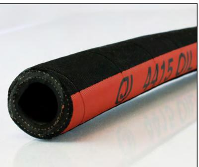
**CONSTRUCTION:** Tube is nitrile, black and smooth, ARPM Class A. Cover is CR, black, ARPM Class B. Reinforcement is a two-ply synthetic fabric with a wire helix.
