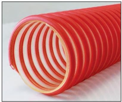
**CONSTRUCTION:** Polyurethane tube with a sturdy clockwise PVC helix with  $S\Omega$  ground wire embedded into the hose wall. TEMPERATURE: -40°F (-40°C) to +140°F (+60°C)
