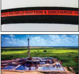
**CONSTRUCTION:** Tube is a nitrile blend blend. Cover is an NBR/PVC blend. Reinforcement is a 4-ply high-tensile synthetic textile with a single wire helix. Dual wire helix for 8", 10" and 12" I.D.'s. and has an anti-static copper wire.
