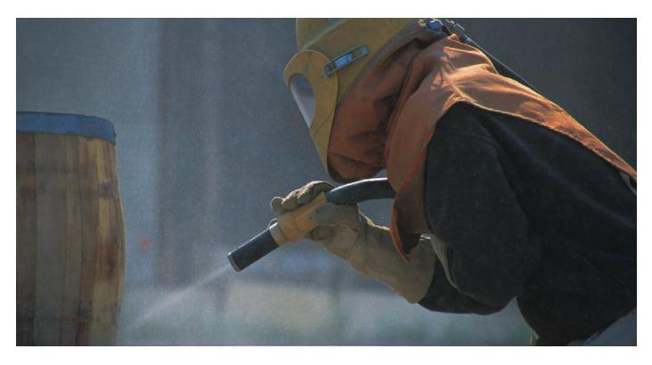
The flow of certain materials inside of a hose can cause a dangerous static charge to build up. When the static charge reaches a sufficient level, it can shock or create an electrical discharge which can lead to fire and explosions.
