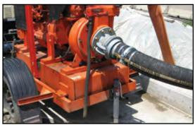
CONSTRUCTION: Tube and cover are an EPDM/SBR
