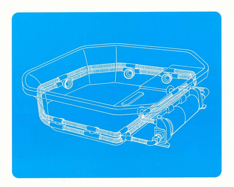
Flexible Kanaflex Pool and Spa Hose can eliminate the need for half the fittings used on your spas. This means you can reduce direct labor time and lower overall cost for assembly while actually improving the quality of the plumbing on your spas.
