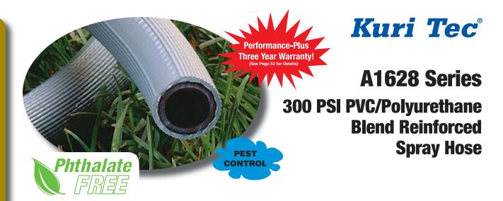
Unique PVC/polyurethane blended core provides excellent resistance to hydrocarbon-based lawn care and pest control chemicals. Reinforced with high tensile strength yarn. PVC ribbed cover provides abrasion resistance.
