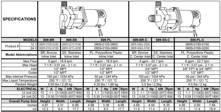
All specifications & data are based on pumping water & are intended as a guideline only. Specifications may vary with different motors.
