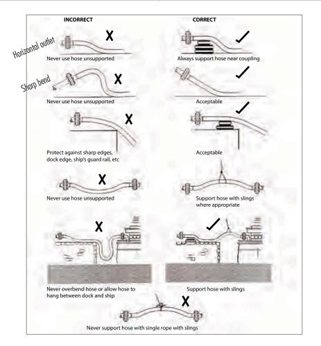
Use a **BEND RESTRICTOR** to prolong hose life when hose is used on horizontal outlets or sharp bends. (See also page 6) **Note:** Due to the inherent nature of composite hose it is susceptible to stretching in length while pressurized. Hose elongation while under pressure is not an indication of failure of films and fabrics. It is therefore critical that this be taken into consideration when calculating the overall length for a hose assembly in operation.
