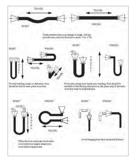
Hose should never be placed into an application that induces twist, rotation or torques the hose.
